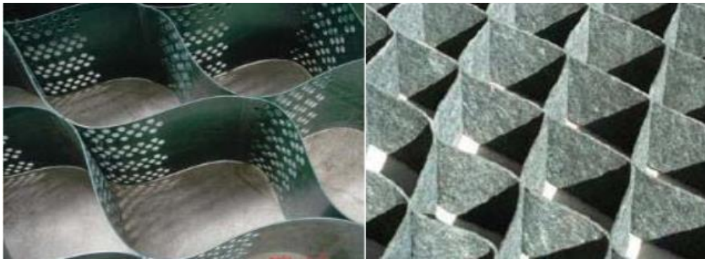
Figure 2: Geocell composition: (a) High density polyethylene; (b) Polypropylene.
