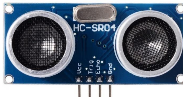
Figure 3 A low-cost ultrasonic distance measuring sensor [11]
