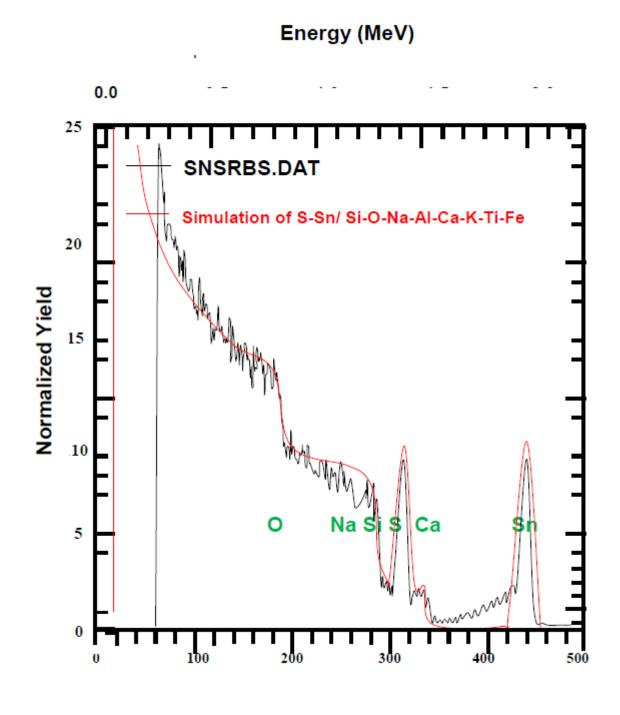
LAYER Thickness Sublayers Channel Composition ... 1 100.00 nm auto Sn 0.501 S 0.499
