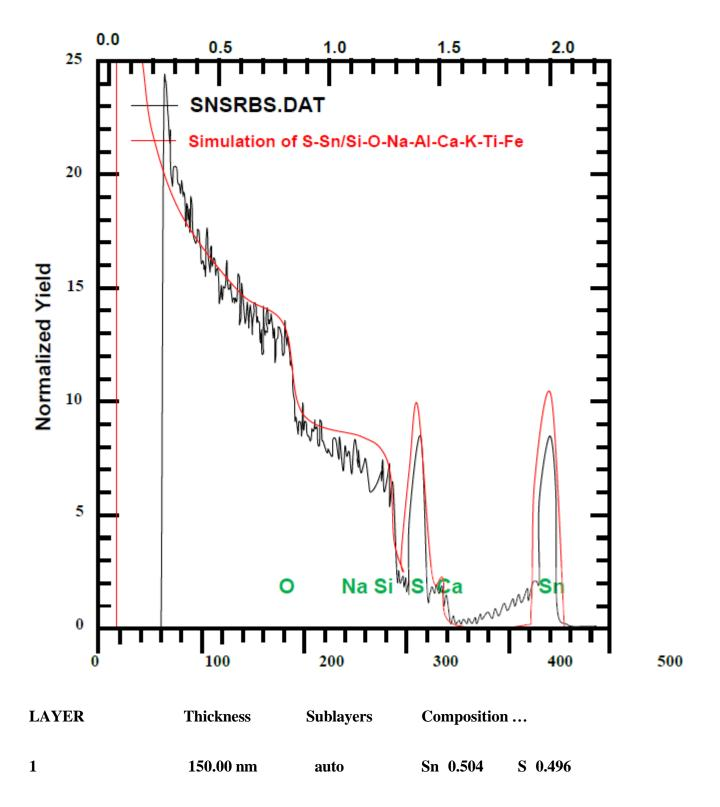
The thickness of the films are 100.00nm for 3hours and 150.00nm for 1hour and the percentage compositions of Tin (Sn) is 50.1% and Sulphur (S) is 49.9 % for 3hours and Tin (Sn) is 50.4% and Sulphur (S) is 49.6% for 1hour sample.
