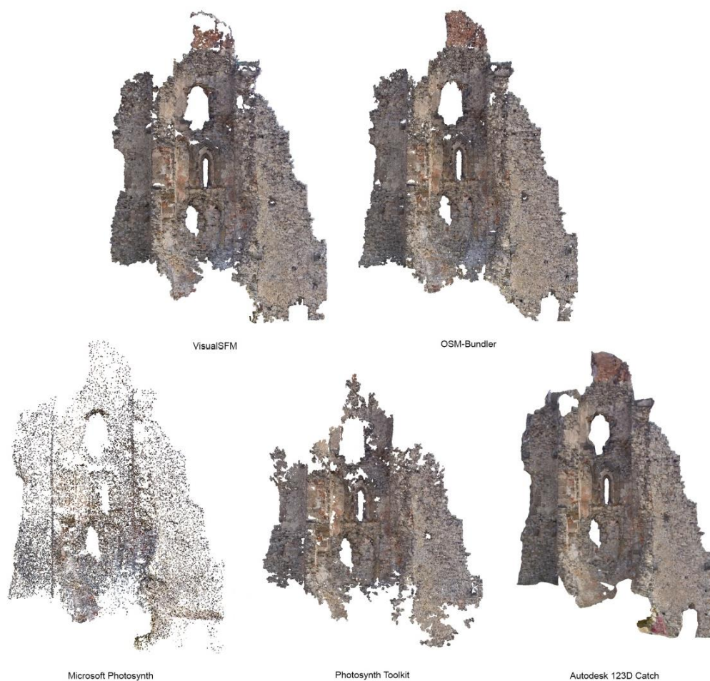
Figure 5: Example of point clouds created from images of object of historical monument using each of tested software [4]
