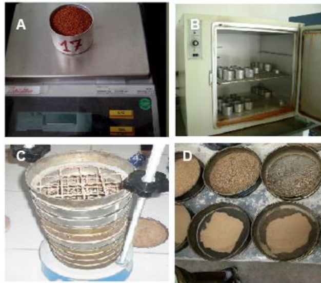
Figure 5. (A) Soil weighing; (B). Soil in the greenhouse; (C and D) Screening test and separation of solids from soil separation
