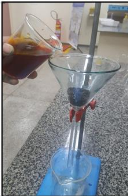
Figure 4 - Analysis of activated charcoal through methyl orange being prepared for spectrophotometry.
