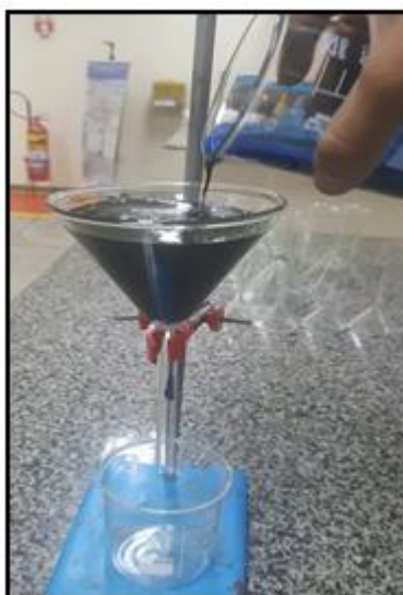
Figure 5 - Activated carbon adsorption analysis through the methylene blue dye filtration.
