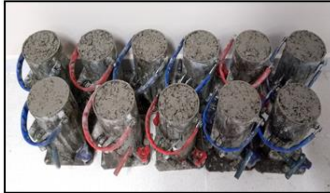
Figure 6 - Newly molded specimens. The front ones (5) are conventional and the rear ones (6) are with activated carbon.
