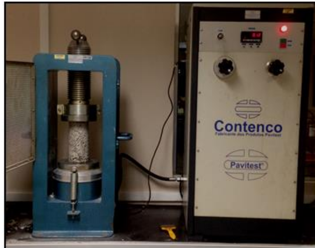
Figure 7 - Specimen positioned awaiting rupture through the digital hydraulic press.
