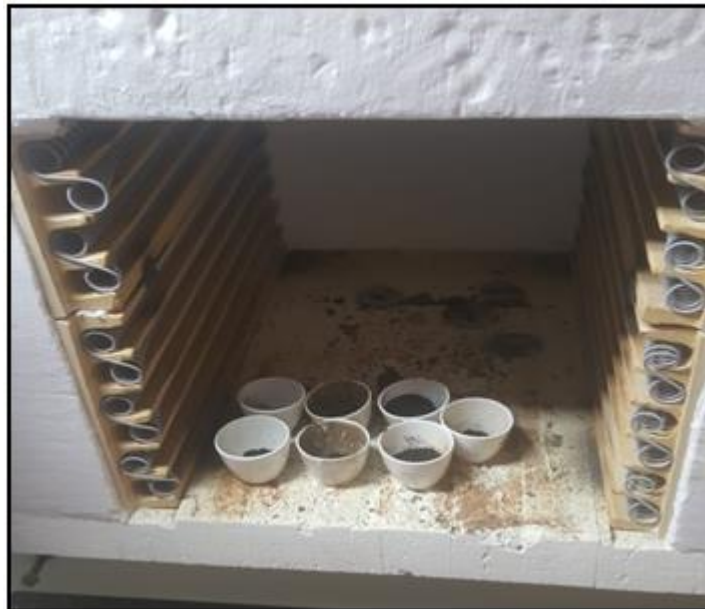
Figure 2 - Combustion of the raw material for the production of activated charcoal.
