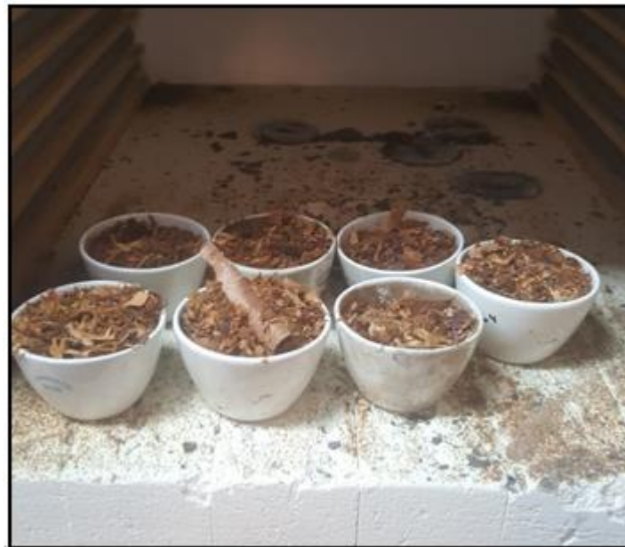
Figure 3 - Activated charcoal production by sawdust combustion inside porcelain containers.
