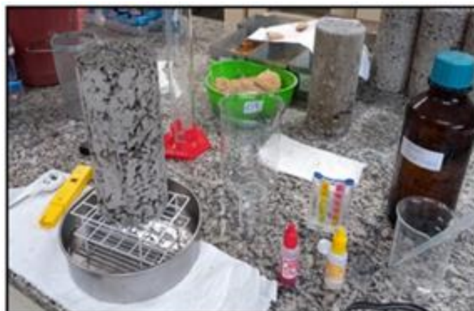
Figure 8 - Materials and equipment arranged on the bench for the filtration of water in the concrete's CPs for analysis.
