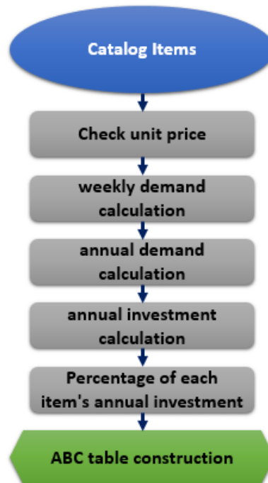
Figure 2: Steps of the ABC Table Build Process
