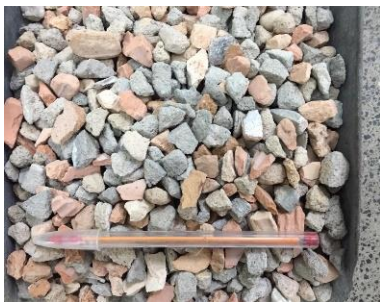
Figure 3 – Graded aggregate - 9.5 mm.
