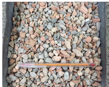
Figure 4 – Graded aggregate - 4.8 mm.
