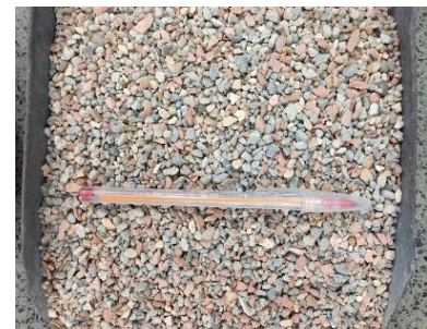
Figure 5- Mud aggregate - 2.4 mm.
