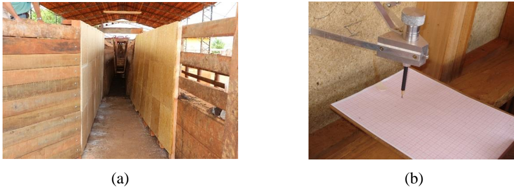
Fig. 4. Bovine management center: (a) Crowding pen internal view. (b) Device to measure horizontal displacement.
