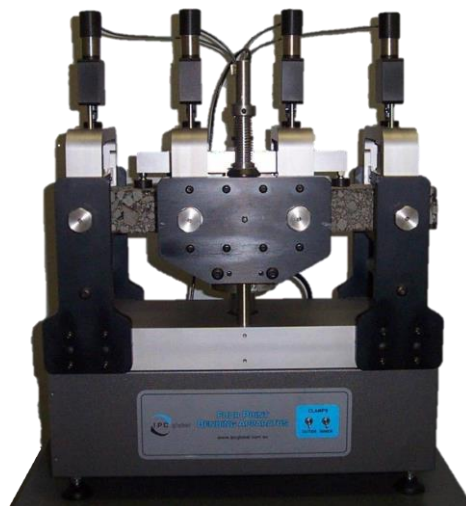
Figure 2: four point bending test equipment.
