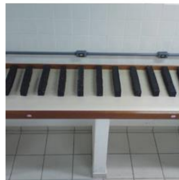
Figure 10. Beams ready for Fatigue Testing
