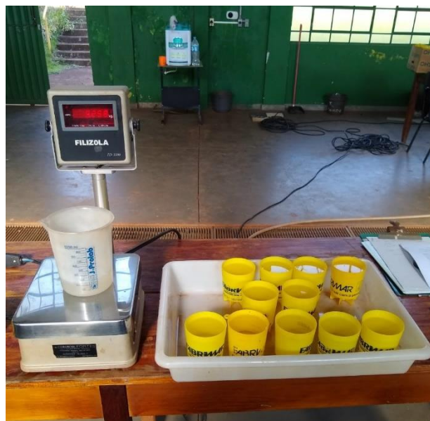
Figure 3. Weighing dripper uniformity test volume.
