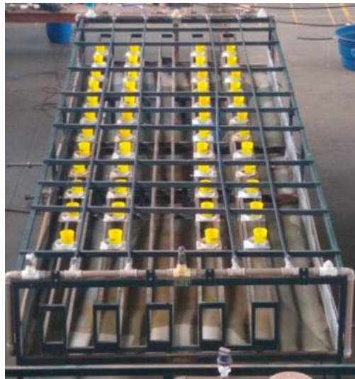
Figure 1. Irrigation Laboratory - Dripper test bench.
