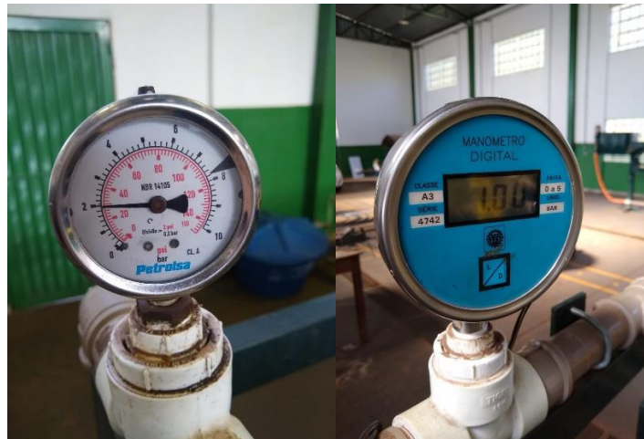
Figure 2. Bourdon type digital and analog pressure gauge.
