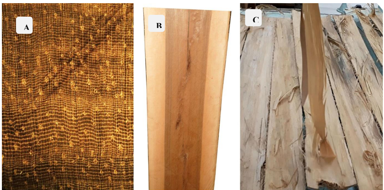
Figure 1- (A) Transversal plane macrophotography (10X); (B) Heartwood and sapwood; (C) Fibrous liber
