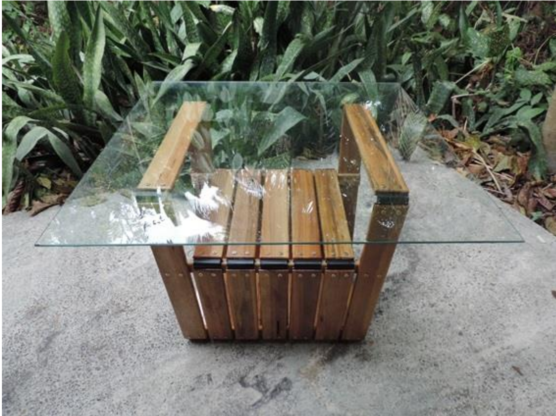
The following processes were used to produce the above piece of furniture: thickening, planing, sanding, lateral tearing, drill drilling and gluing. Figure 4- Coffee table/bench, multifunctional furniture made of E. truncata wood.
