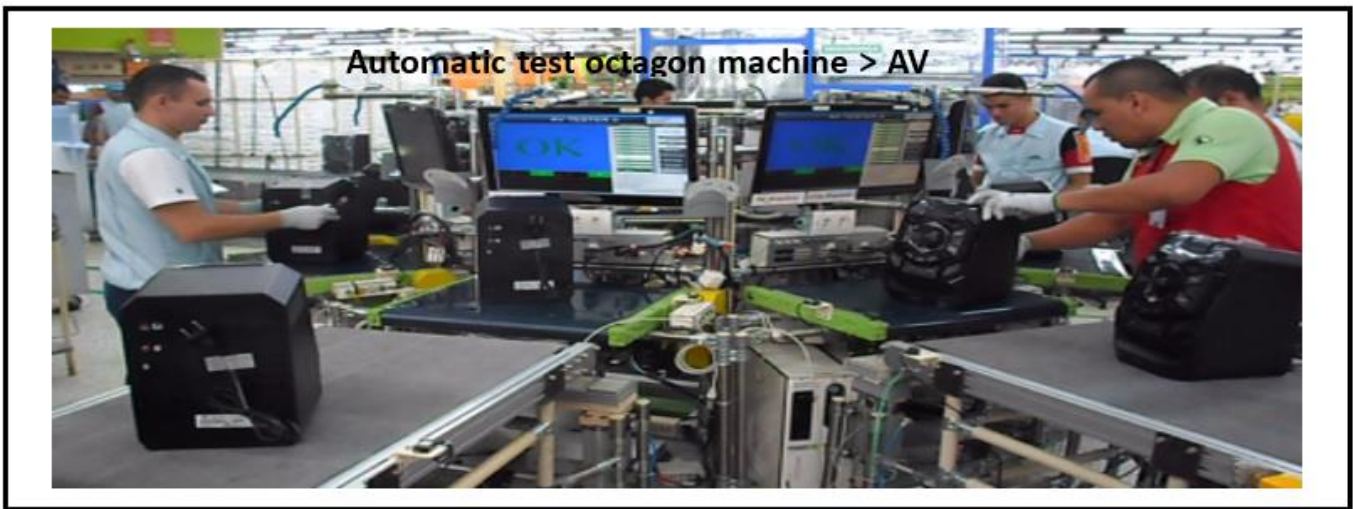
Figure 4: Eight-Sided Carousel Test Cell (After)
