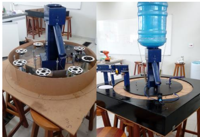
Figure 3 – Final assembly of the conveyor belt with all items attached.
