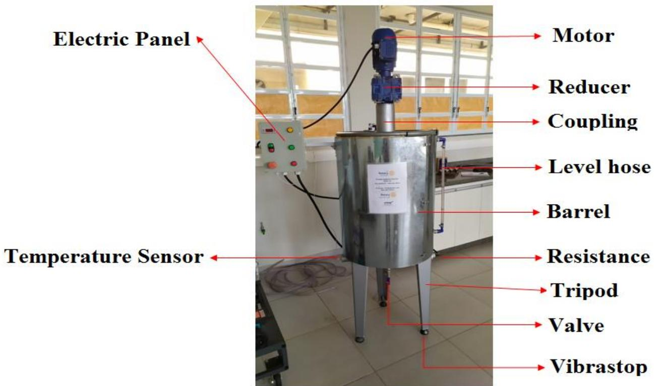
Figure 16. Final reactor system for biodiesel production.
