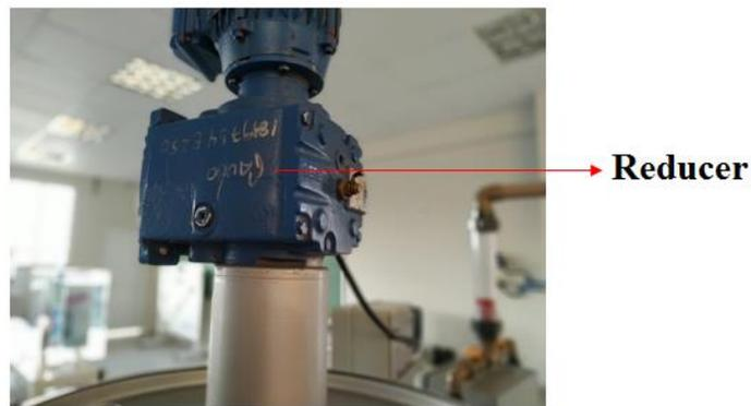
Figure 4. Gear Reduction.
