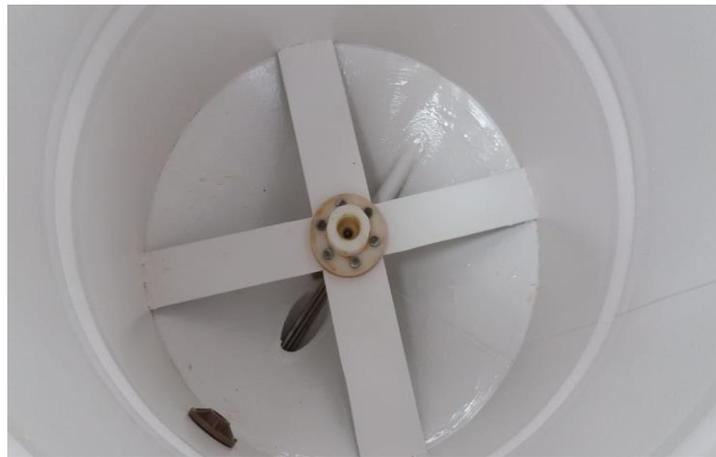
Figure 15. Internally painted reactor drum.
