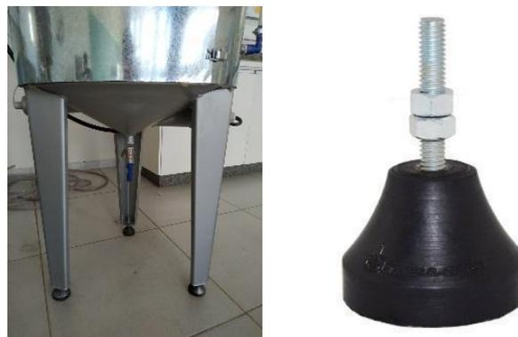
Figure 8. Tripods and dampers for controlling vibrations.
