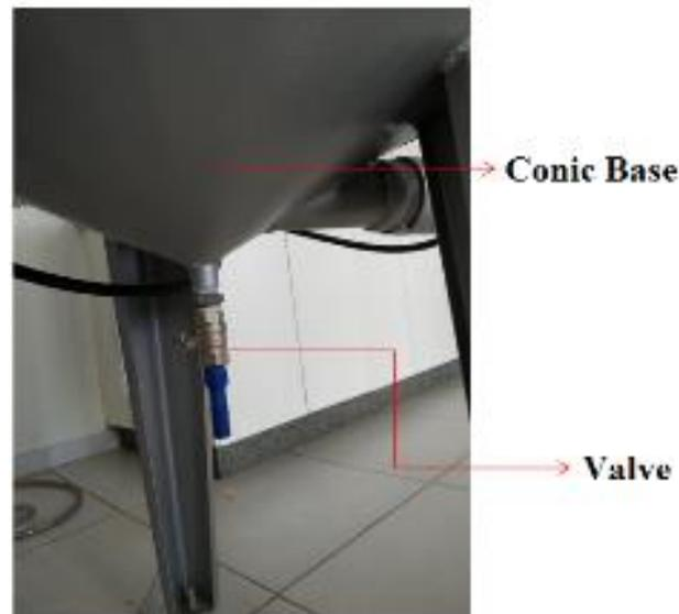
Figure 9. Cone Bottom Tanks and manual flow-control valve.
