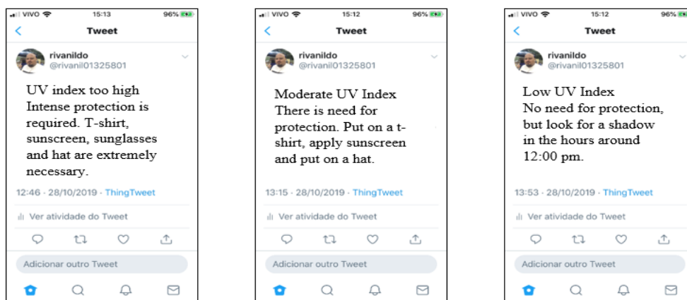
Figure 5. Warning messages about the UV index via Twitter from experiment. Source: ThingSpeak, (2019).
