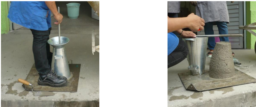
Figure 3 - Concrete abatement test
