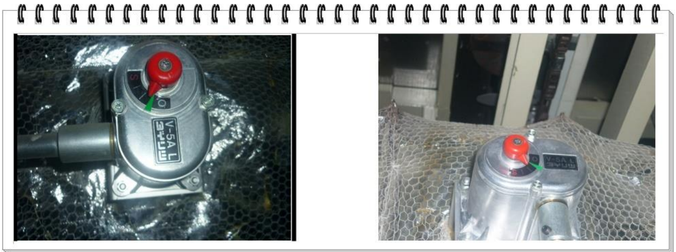
Figura 13: Marking of Flash-off and Exhaust Vent Valves.
