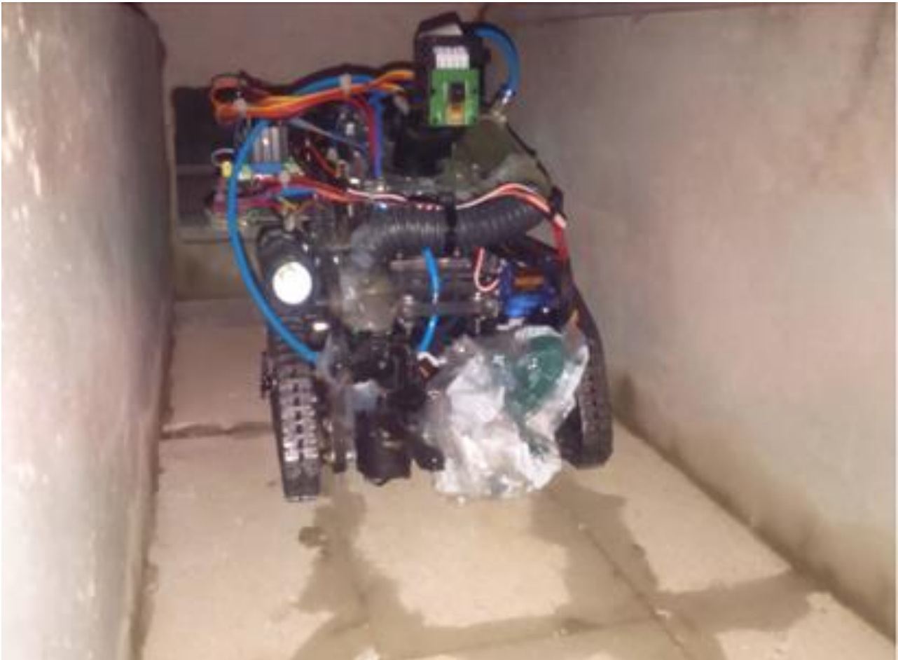
Figure 5. Locomotion by mats in a duct.
