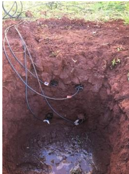
Figure 6. Probe driven at depths of 10 and 30 cm. Dourados-MS, 2020.
