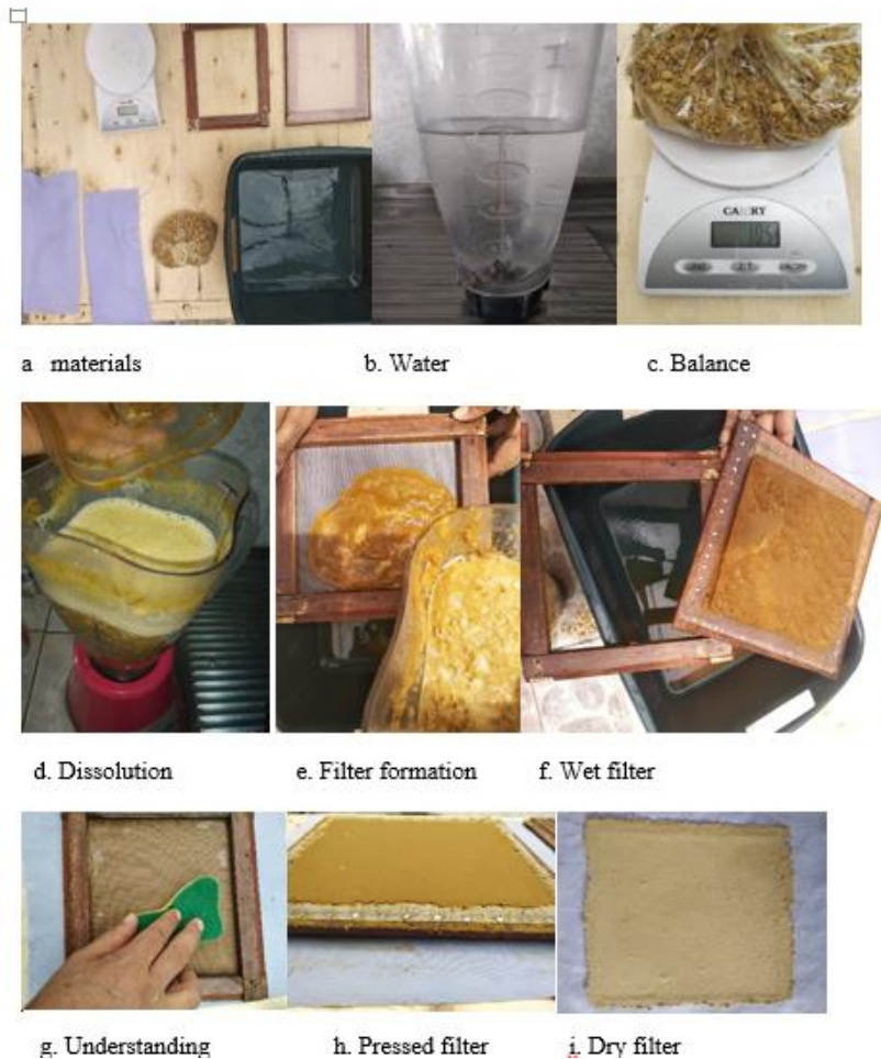
Graph 1. Process for obtaining non-woven (filter) from bamboo cellulose
