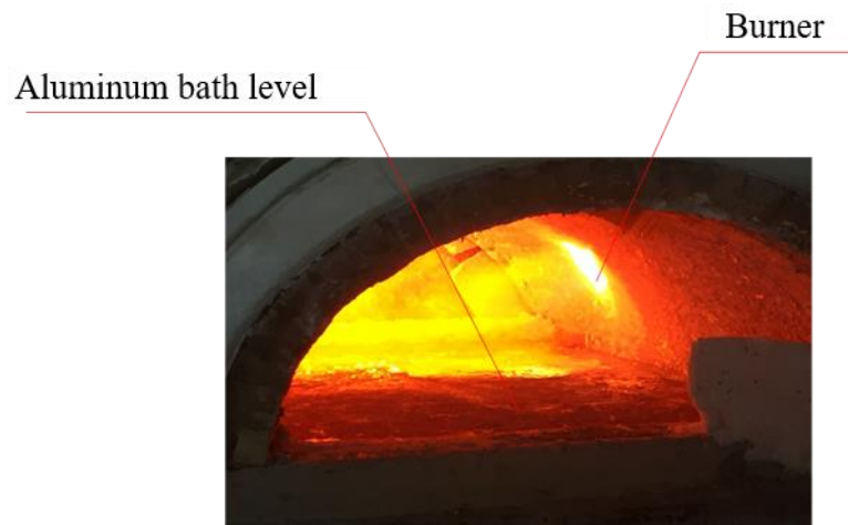
Figure 1: Aluminum bath level flame contact.
