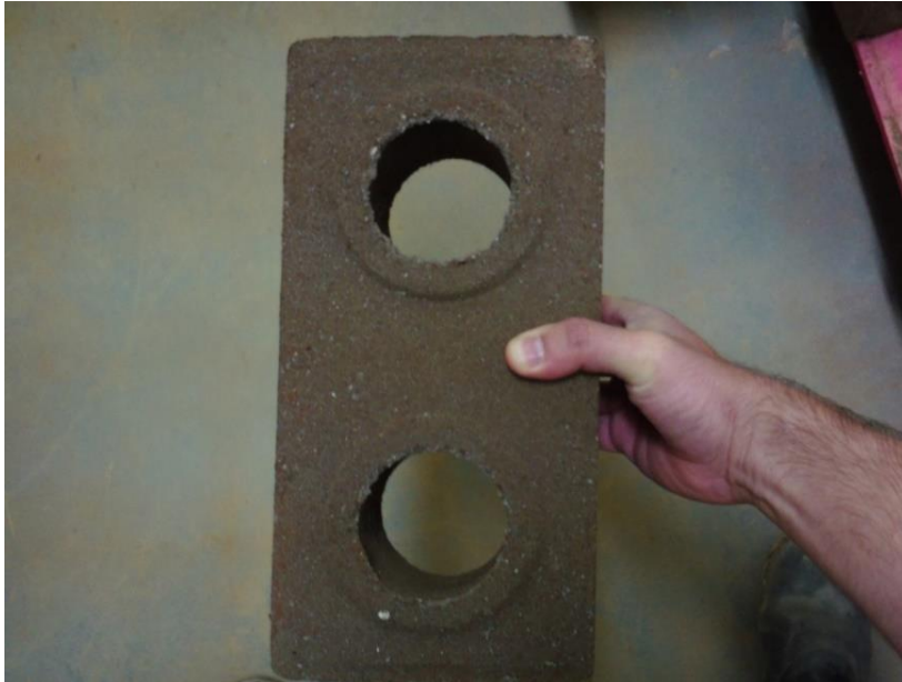
Figure 4 - Ecological Brick with Civil Construction Waste Source: Pinto, 2015
