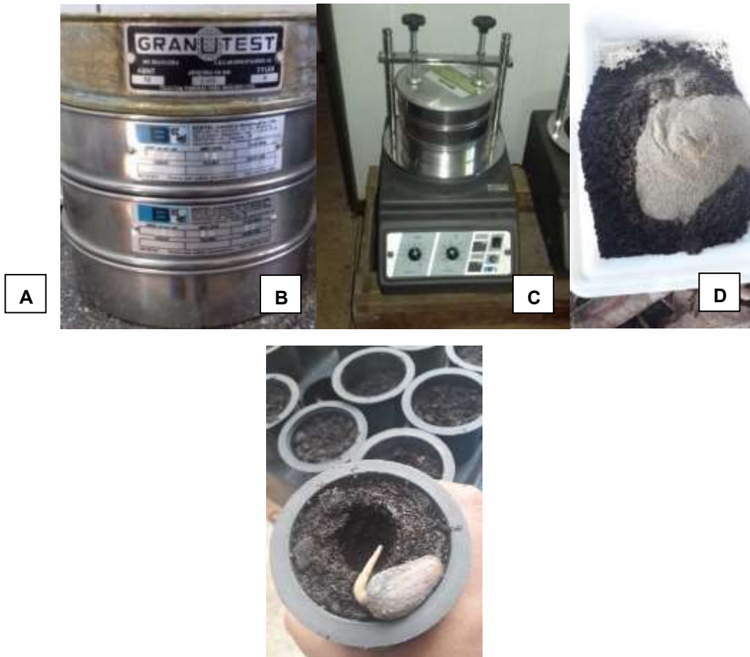
Figure 3: (A) - Sieve in different openings in mm for material preparation; (B) - Digital electromagnetic stirrer making the material sieving; (C) - Rock powder incorporation into the substrate; (D) – Pre-germinated cocoa seeds sowing.
