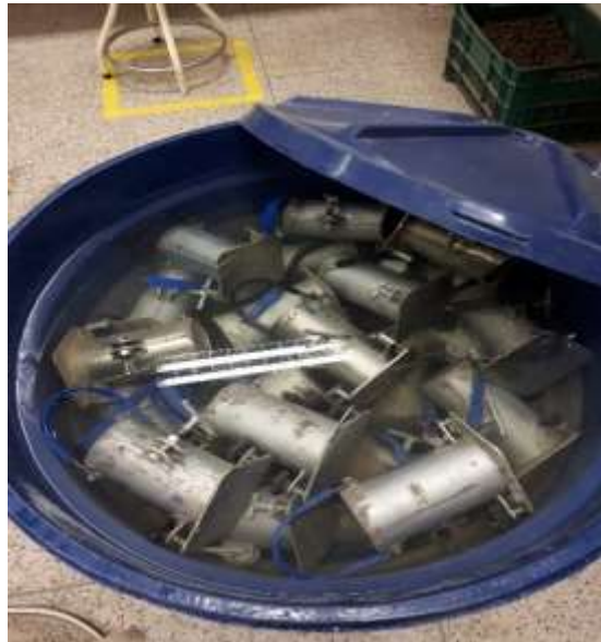
Figure 13: Spicemens submerged in water. Source: AUTHOR (2020).
