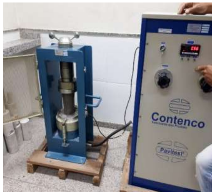
Figure 14: Compression rupture. Source: AUTHOR (2020).
