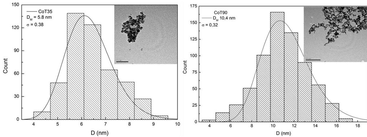
Figure 1. Particle size histogram and the curve fitting using a log-normal distribution function. The inset shows a typical TEM micrograph of samples CoT35, and CoT90.
