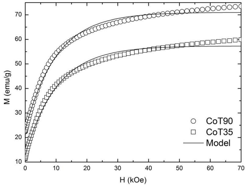
Figure 3. Magnetization loops data (symbols) of two samples (CoT35, and CoT90) and the corresponding curve fitting (solid lines) using a eq. 3.
