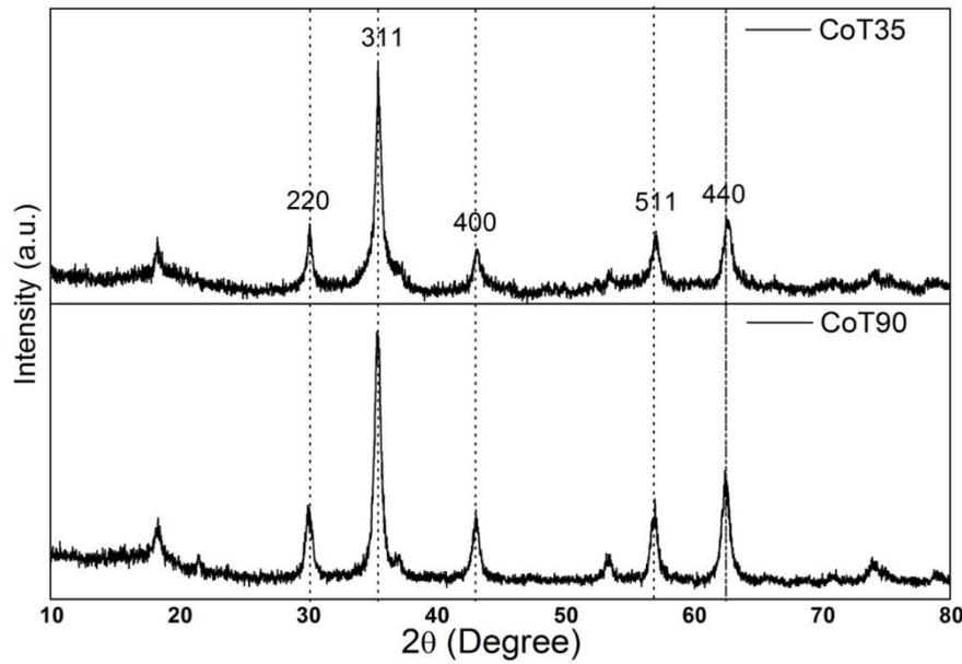
Figure 2. Diffraction pattern of cobalt ferrite nanoparticle of samples CoT35, and CoT90. The average crystallite diameters ( $D_{hkl}$ ) obtained from the (311) XRD peaks of both samples are collect in Table 1.
