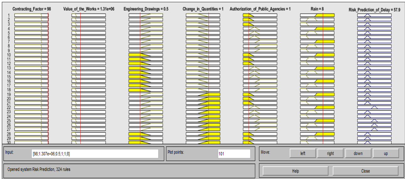
Figure 14. Inference system response for construction 2.
