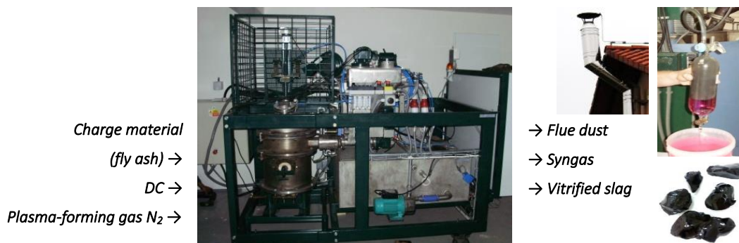
Figure 1. A laboratory plasma reactor; input and output materials [5].
