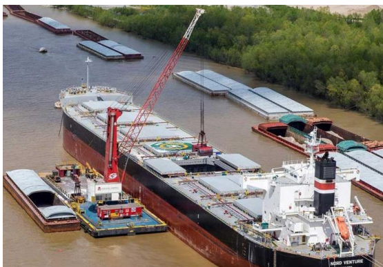
Figure 1. Transshipment with floating crane
