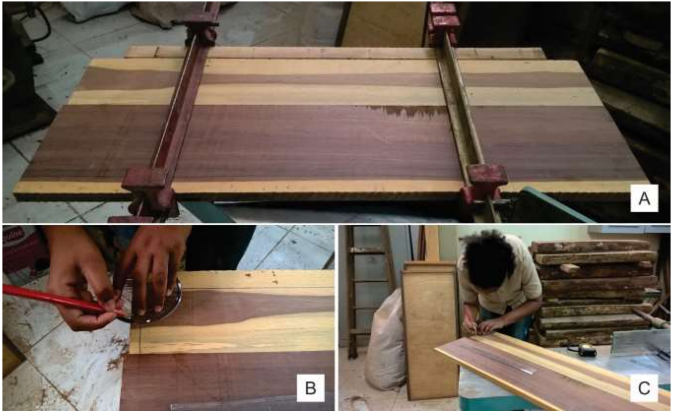
Figure 8. (A) Pressing the parts and (B/C) marking of them for cutting.
