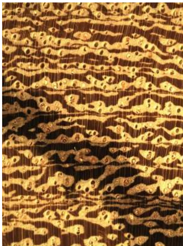
Figure 1. Macrograph of the transversal plane (10x magnification) of Zygia racemosa
