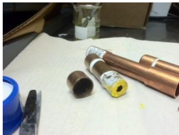
Fig 2. Reusable Custom made copper vials/caps
