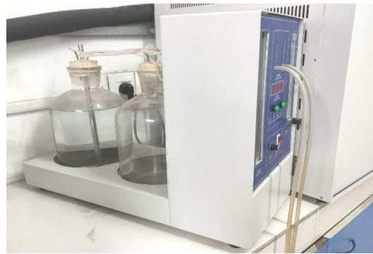
Figure 3. Side view of cold filter point suction device
