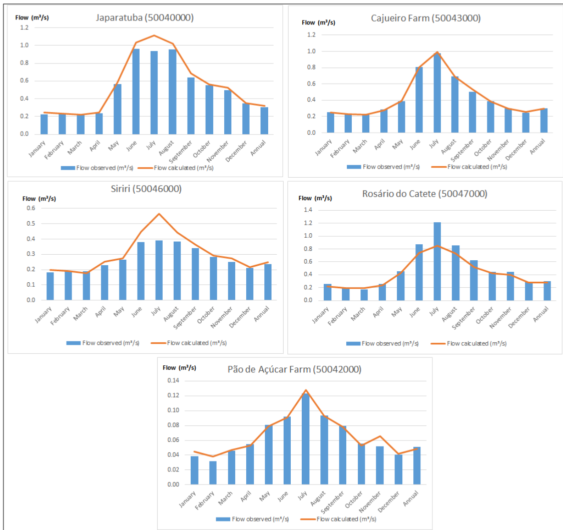
Figure 2. Observed and calculated flow rates for HRI and HR II river stations
