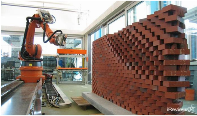
Figure 2. Semi-automated mason (SAM)
