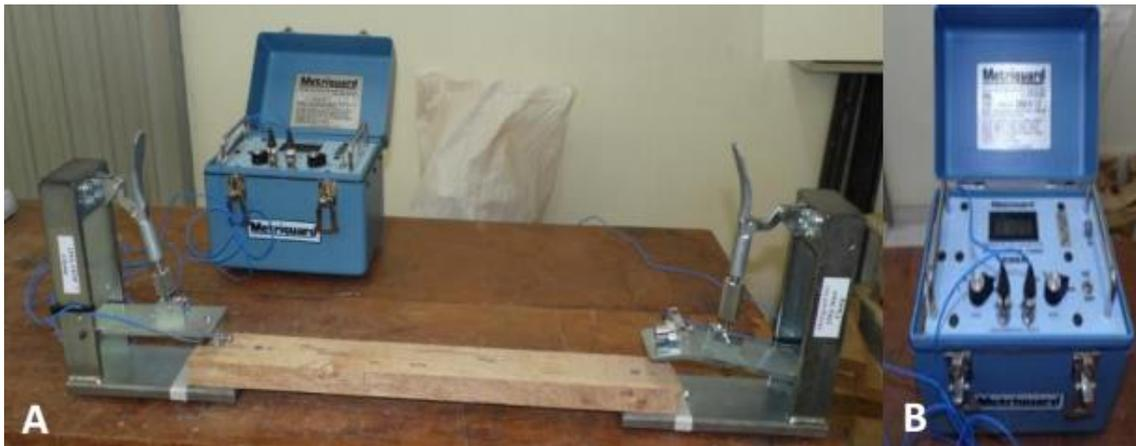
Figure 01: Stress wave timer. A-Sample tested; B-Detail of the equipment
