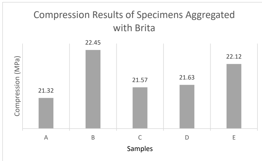
Figure 6. Compression results of aggregated concrete with gravel.
