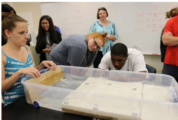
Figure 6. Students measure the wave height at three places along the side of the wave tank.
