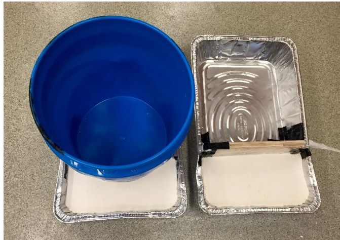
Figure 1. Formation of curved and straight coastline with plaster of paris in tin pans.
