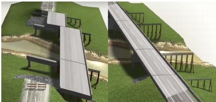
Figure 24 the Second Stage of the Sliding Approach (GarverUSA)
