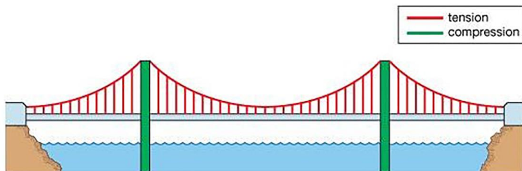
Figure 4 Suspension Bridge (infovisual.info)
