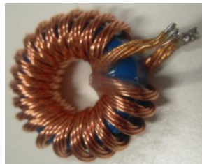
Fig. 11 Photo of inductor, made by student
