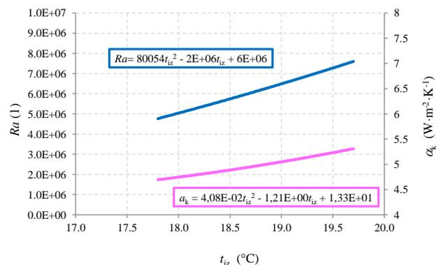
Figure 1. The progress of Rayleigh’s number and the heat transfer coefficient on the outer side of the pipe depends on the change in water temperature for DN125
