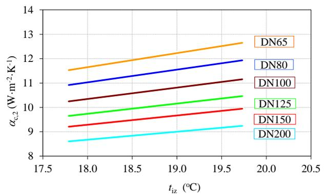
Figure. 5 The progress of the total heat transfer coefficient on the outer side of the tube , depending on the change in the pipe diameter at the constant flow
