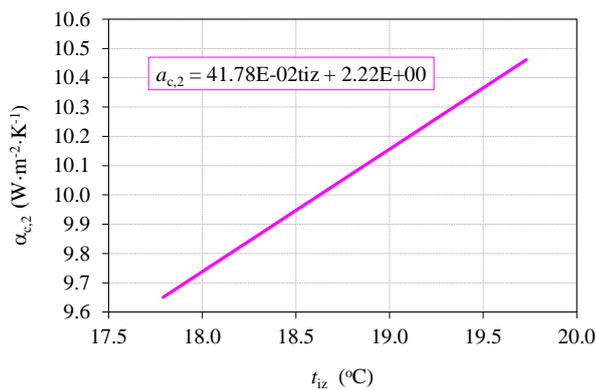
Figure. 4 Progress of  $\alpha_{c,2}$  depending on surface temperature insulation for DN 125
