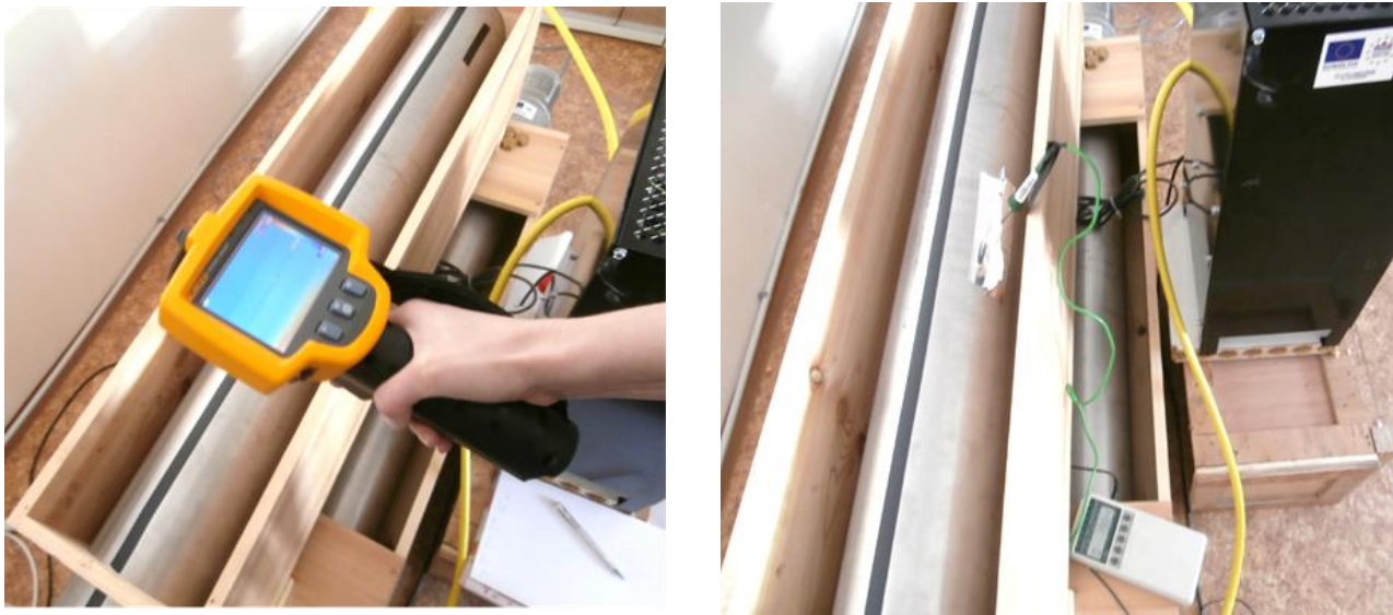
Figure 4. Measurement of the temperature of the metal hydride tank.
