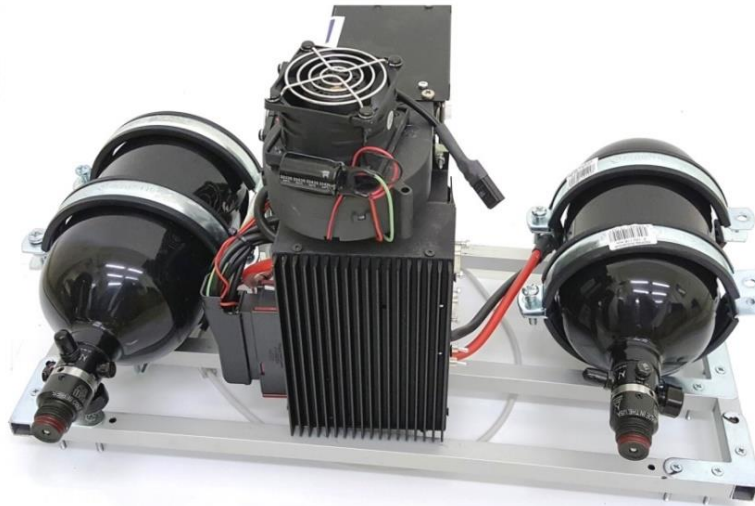
Figure 3. PEM fuel cell and metal hydride tanks with the attachment.
