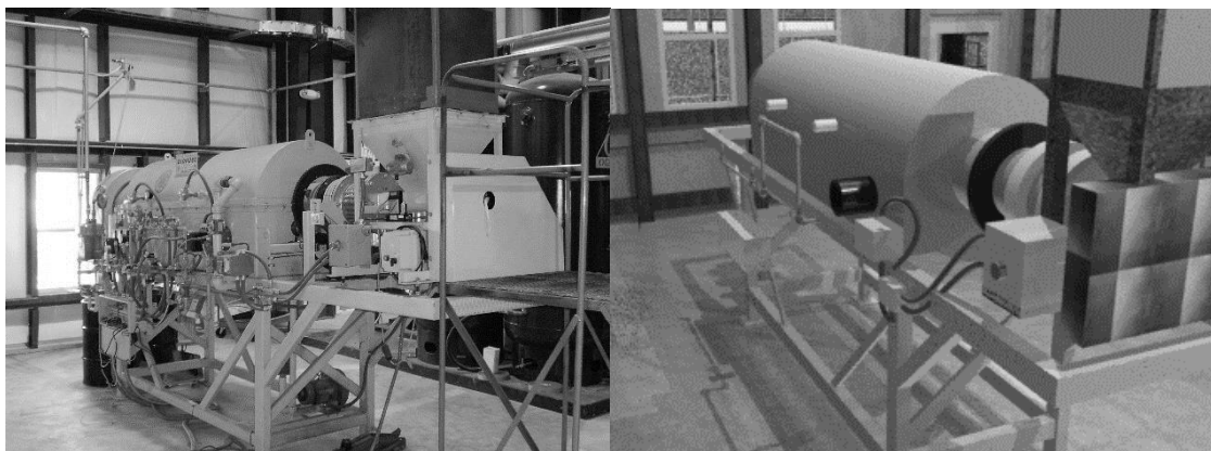
Figure 1: Torrefraction unit and 3ds Max Design rendered model of the unit.
