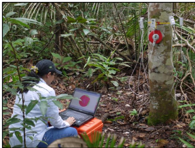
Figure 2: Application of the pulse tomograph to the tree stem.
