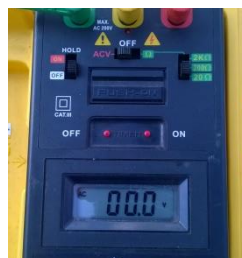
Figura 01 – Terrometer Minipa MTR 1520D.
