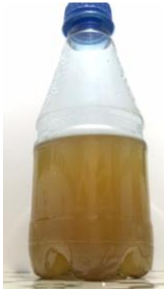
Figure 4 - Oil obtained by the pyrolysis process.
