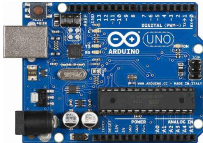
Figure 2. Uno arduino plate. SOURCE: ARDUINO cc, 2019
