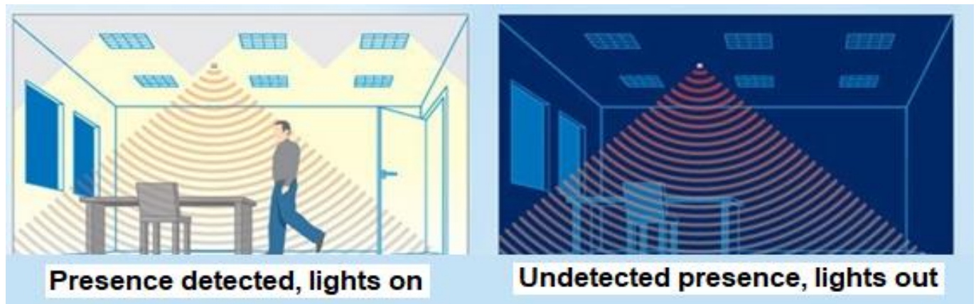
Figure 1 - Detection area of the presence sensors.
