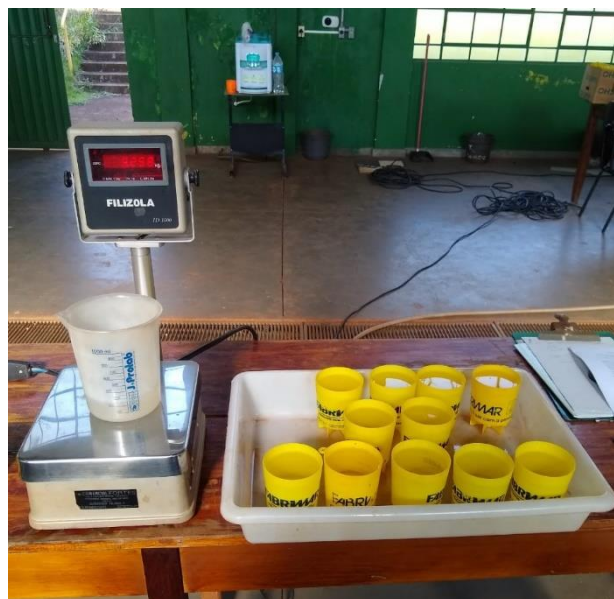
Figure 3. Weighing dripper uniformity test volume.
