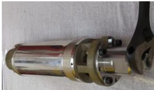
Figure 13 - Hexagonal Center Flange Coupled to Pump
