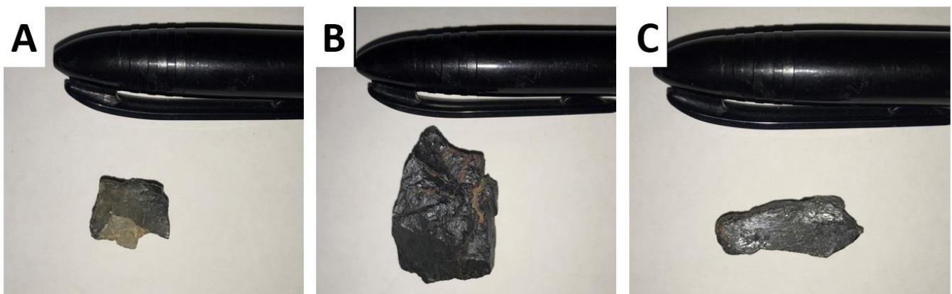
Figure 10. A. Quartz grain. B. Hematite. C. Ilmenite. All from sample A01-R.
