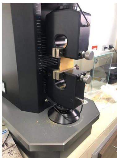
Graph 2. Bamboo Nonwoven (Filter) Strength and Expansion Test
